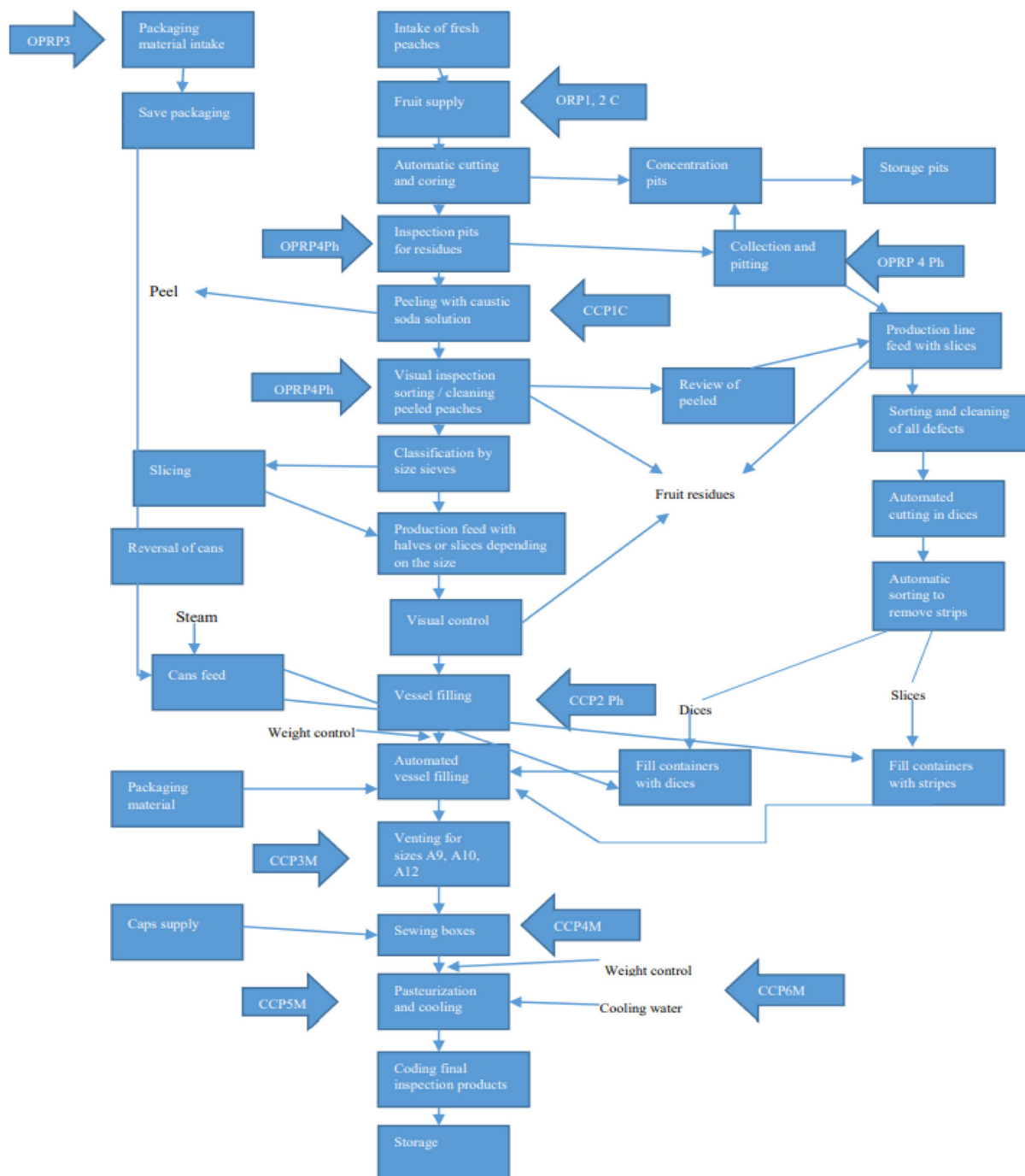
Figure 8. Production Flowchart of a Food Canning Company
